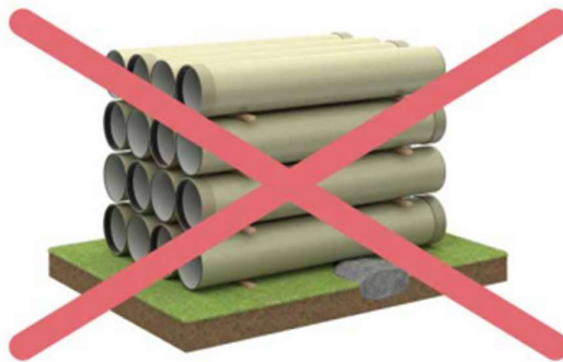
Figure 6 – Pipes Should not Rest on Stones
