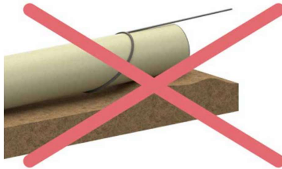
Figure 8 – Pipes Should not be Dragged along the Ground
