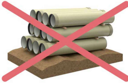
Figure 7 – Pipes Should not Rest on Uneven Surface
